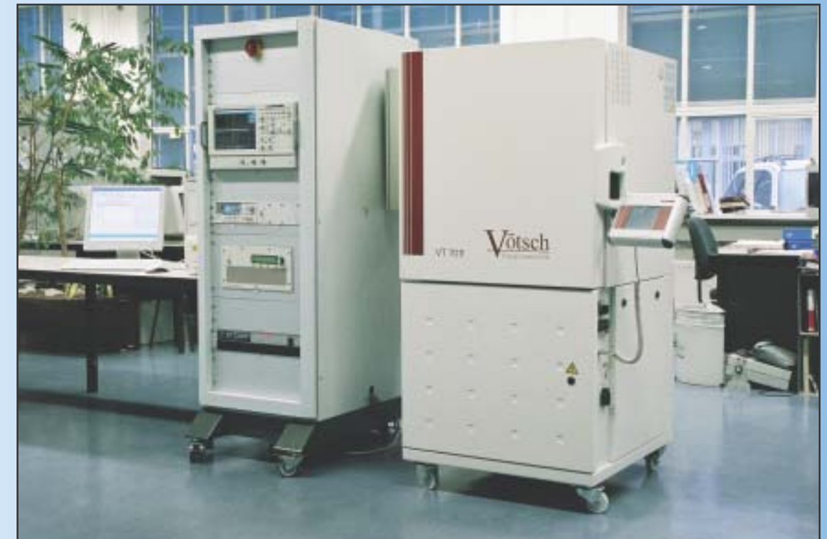
Powerless measurement setup for ferrites
