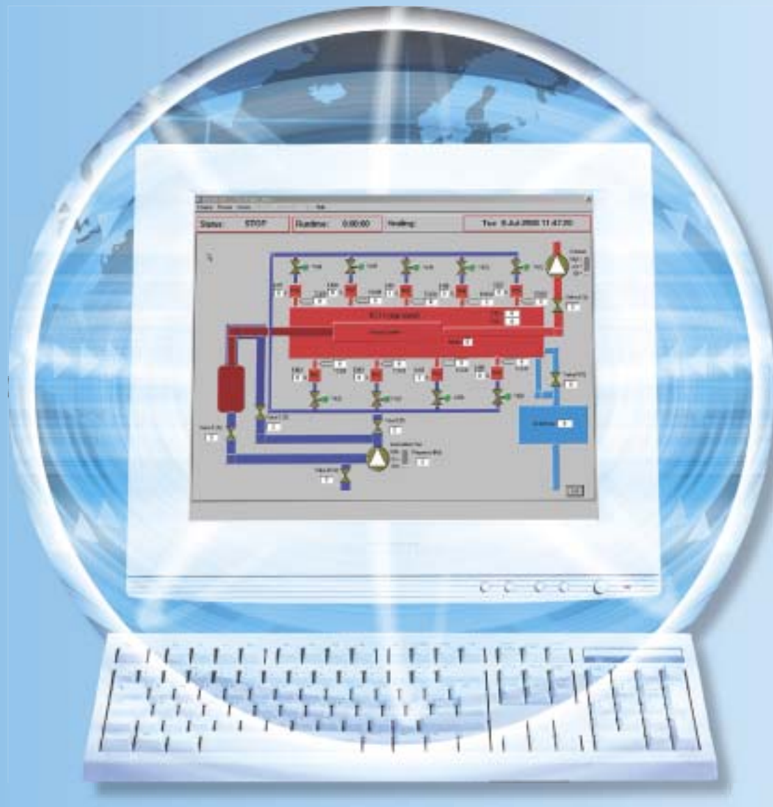
Kiln control system screen snapshot
