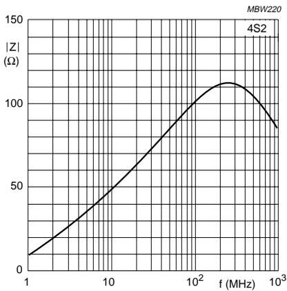
Fig.4 Impedance as a function of frequency,
