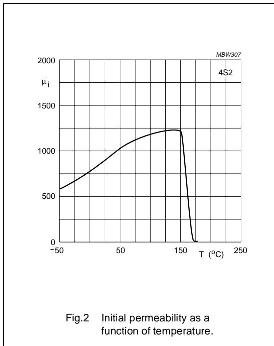
Fig.2 Initial permeability as a function of temperature.
