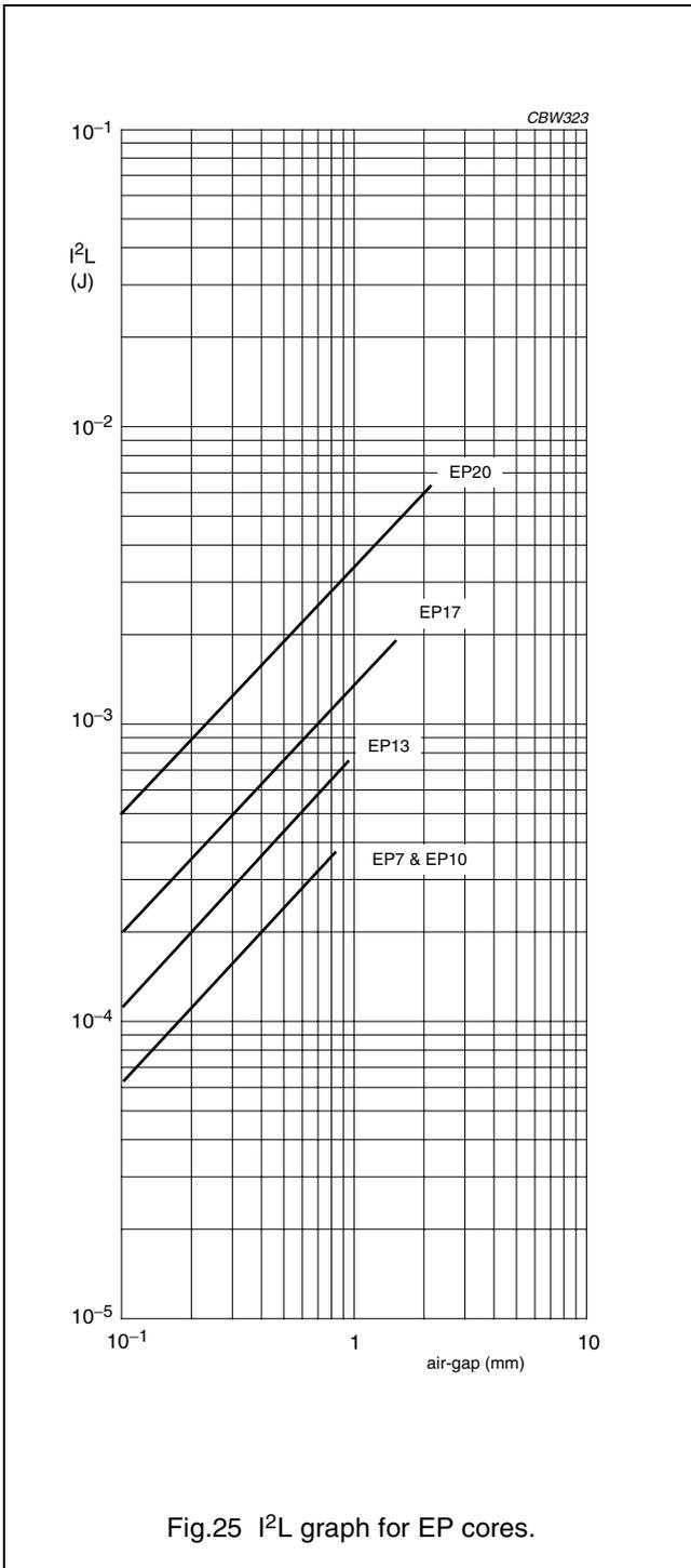
Fig.25  $I^2L$  graph for EP cores.
