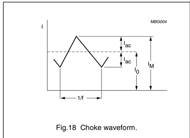
Fig.18 Choke waveform.
