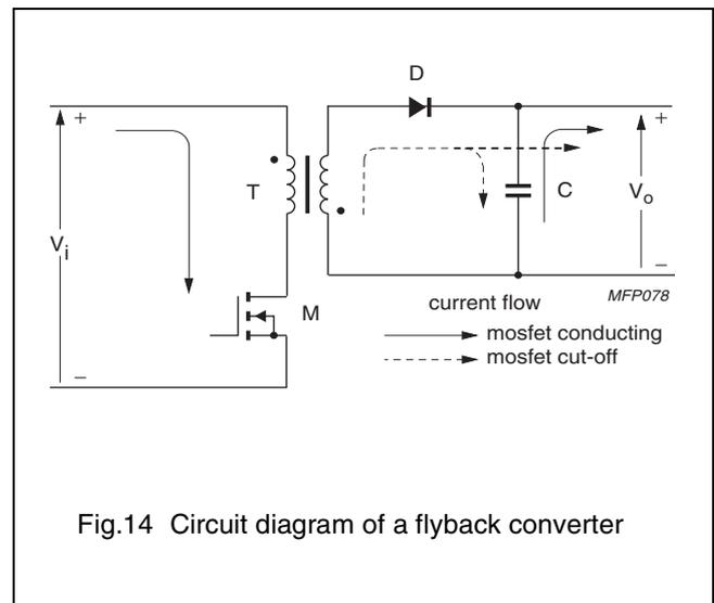
Fig.14 Circuit diagram of a flyback converter
