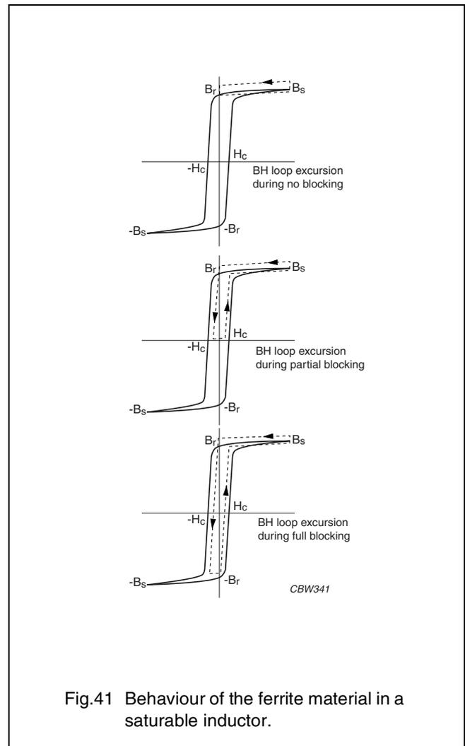
Fig.41 Behaviour of the ferrite material in a saturable inductor.
