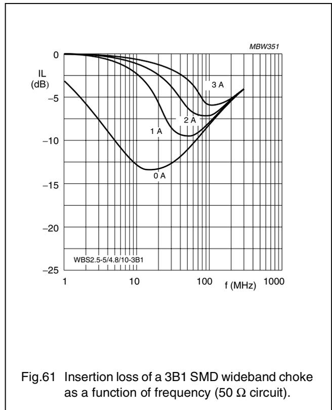
Fig.61 Insertion loss of a 3B1 SMD wideband choke as a function of frequency (50 Ω circuit).
