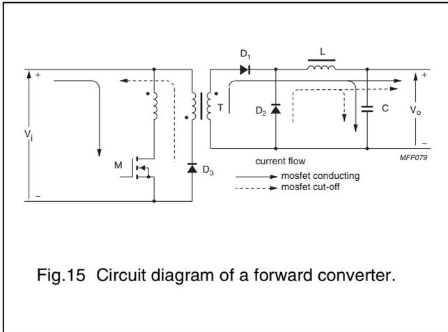
Fig.15 Circuit diagram of a forward converter.
