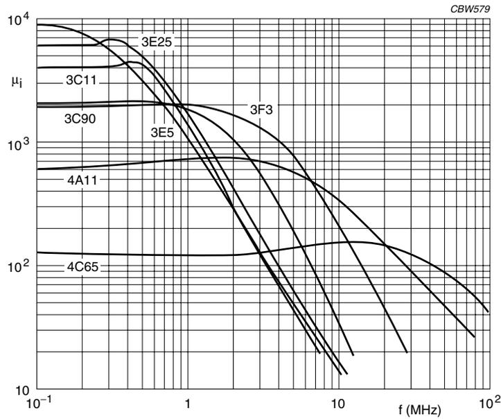
Fig.39 Permeability as a function of frequency of different materials.
