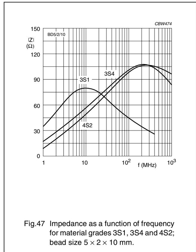
Fig.47 Impedance as a function of frequency for material grades 3S1, 3S4 and 4S2; bead size  $5 \times 2 \times 10$  mm.
