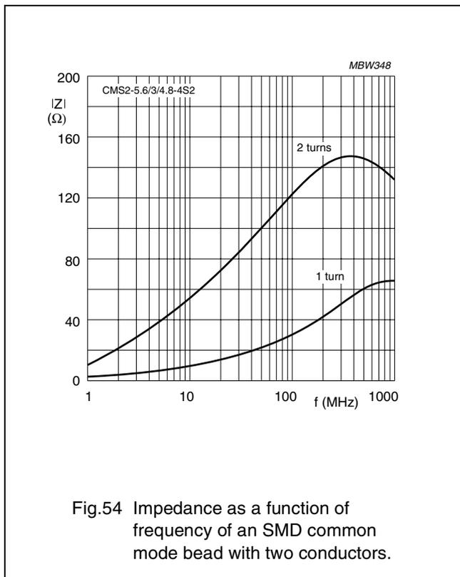
Fig.54 Impedance as a function of frequency of an SMD common mode bead with two conductors.
