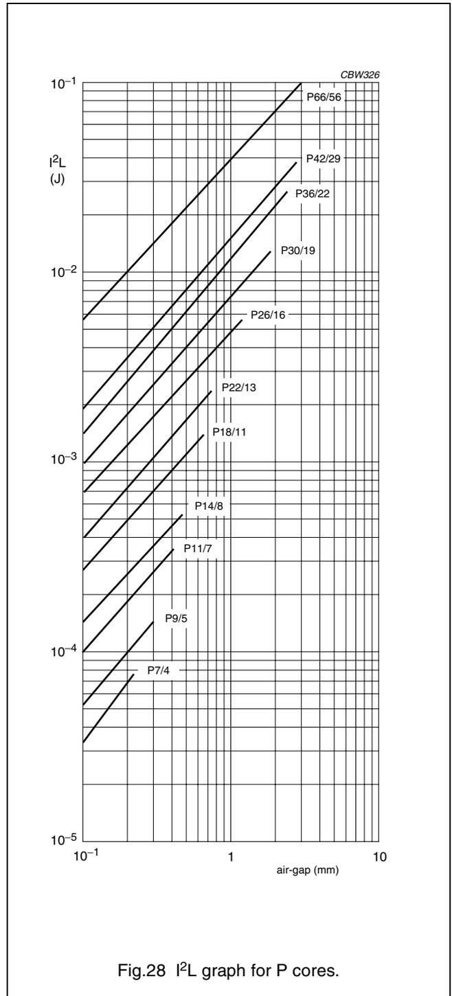
Fig.28  $I^2L$  graph for P cores.
