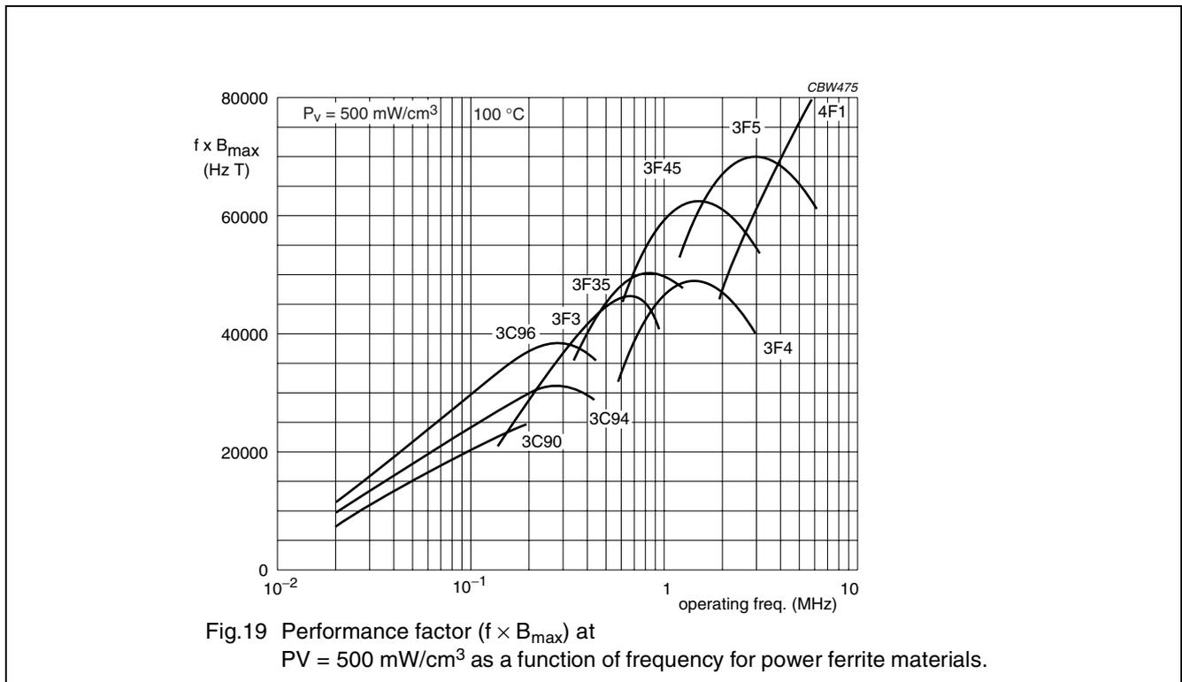
Fig.19 Performance factor ( $f \times B_{max}$ ) at  $PV = 500 \text{ mW/cm}^3$  as a function of frequency for power ferrite materials.
