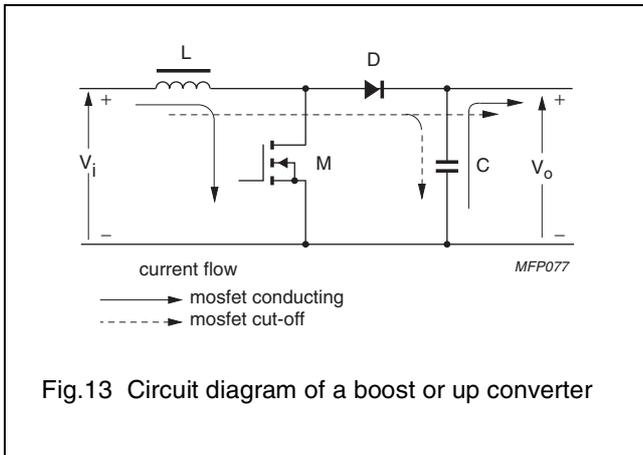
Fig.13 Circuit diagram of a boost or up converter
