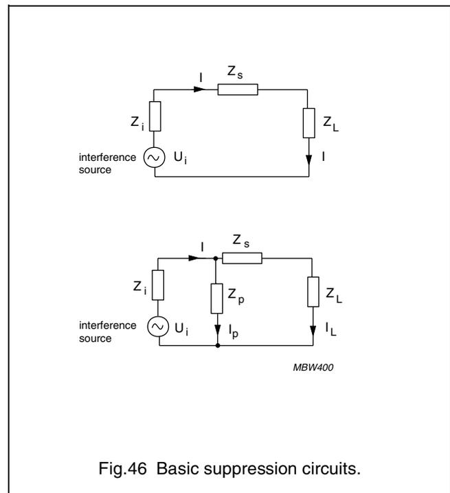
Fig.46 Basic suppression circuits.
