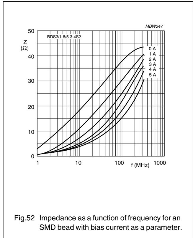
Fig.52 Impedance as a function of frequency for an SMD bead with bias current as a parameter.
