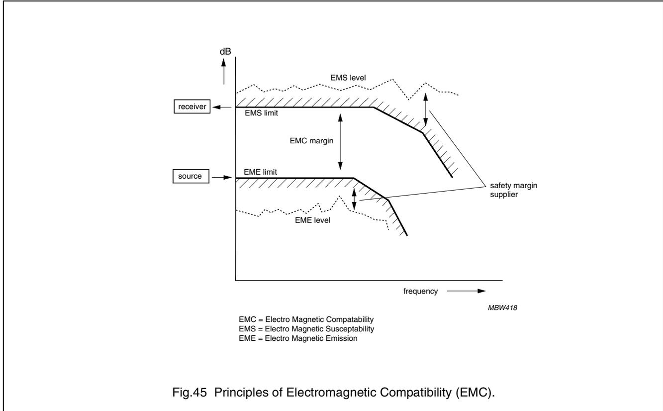
Fig.45 Principles of Electromagnetic Compatibility (EMC).
