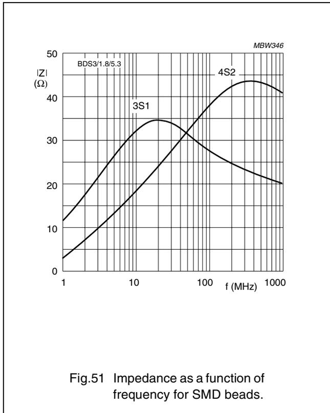
Fig.51 Impedance as a function of frequency for SMD beads.
