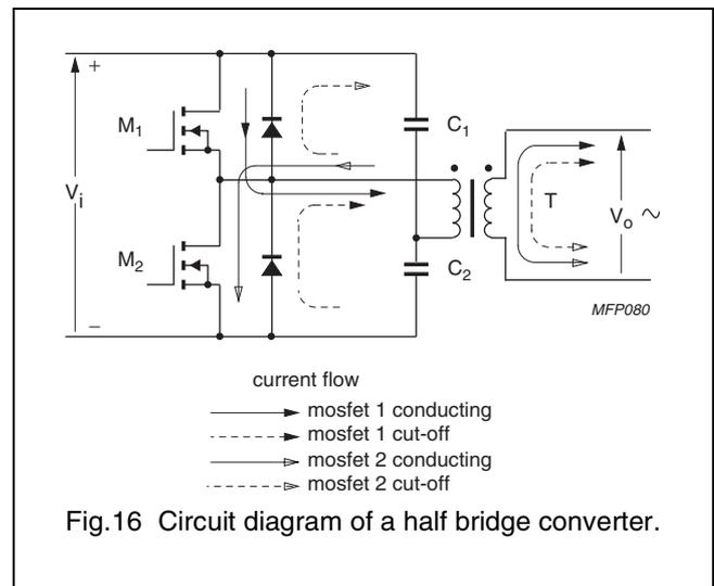
Fig.16 Circuit diagram of a half bridge converter.
