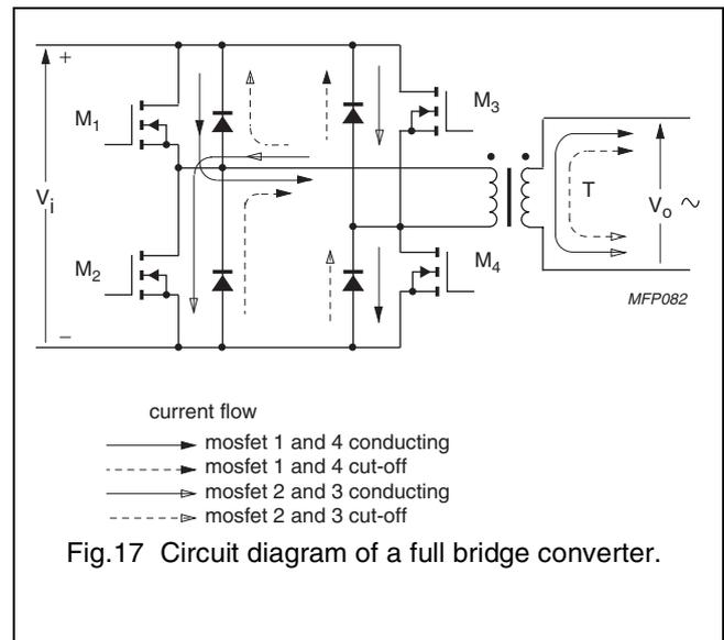
Fig.17 Circuit diagram of a full bridge converter.
