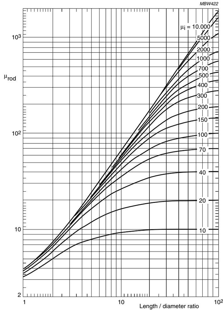
Fig.64 Rod permeability ( $\mu_{rod}$ ) as a function of length to diameter ratio with material permeability as a parameter.
