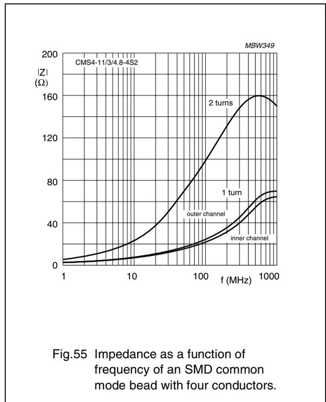
Fig.55 Impedance as a function of frequency of an SMD common mode bead with four conductors.
