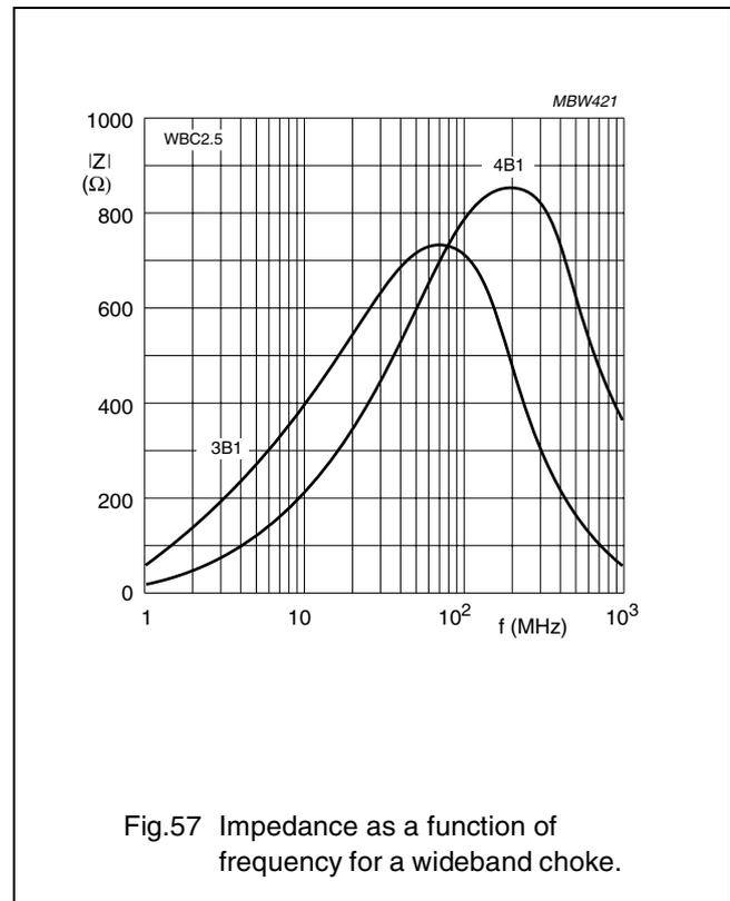
Fig.57 Impedance as a function of frequency for a wideband choke.
