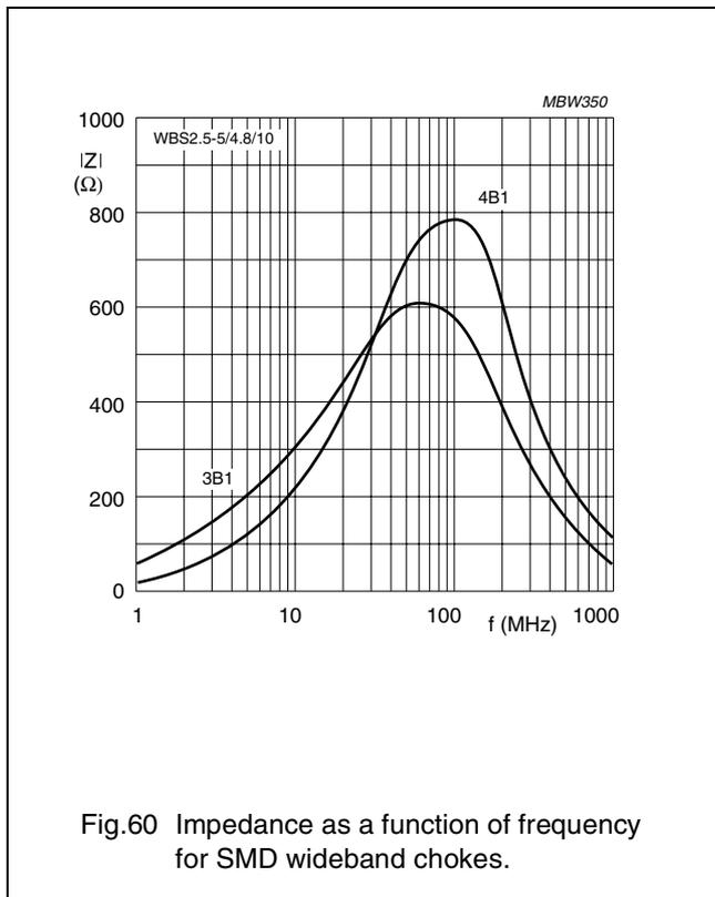
Fig.60 Impedance as a function of frequency for SMD wideband chokes.
