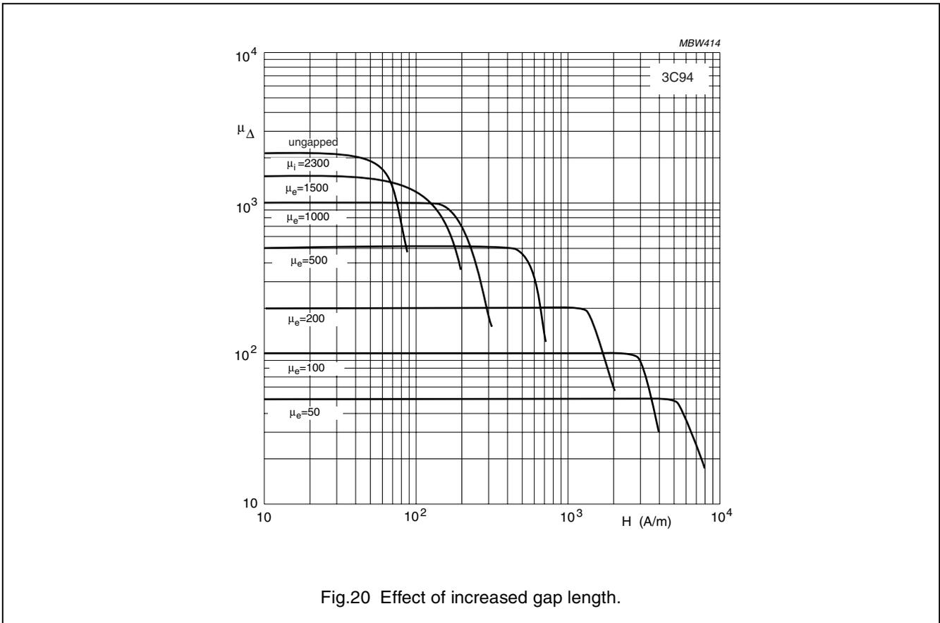
Fig.20 Effect of increased gap length.
