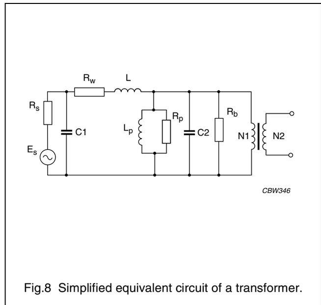
Fig.8 Simplified equivalent circuit of a transformer.
