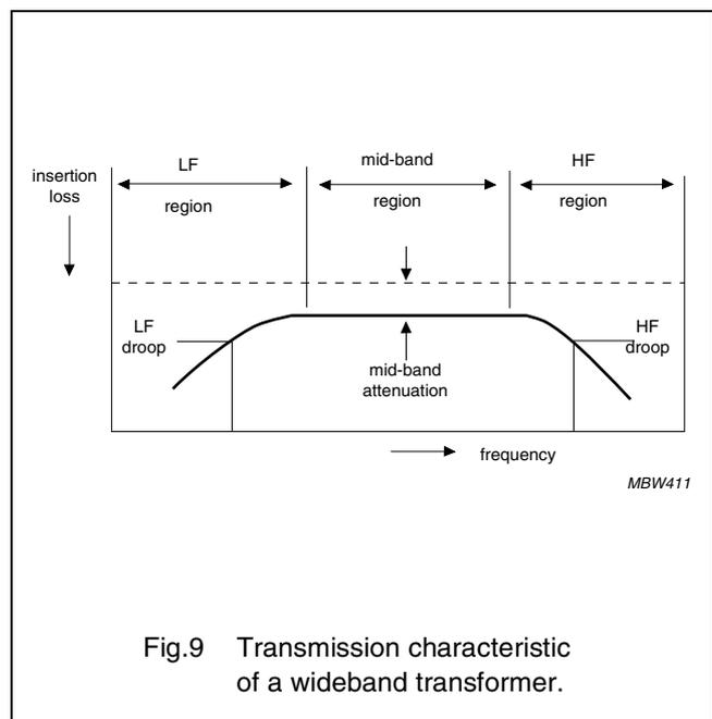
Fig.9 Transmission characteristic of a wideband transformer.
