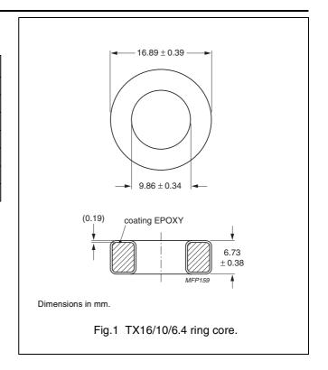
Ring core data - Note 1. Mechanical dimensions : OD  $\leq$  17.4, ID  $\geq$  9.53, H  $\leq$  7.11
